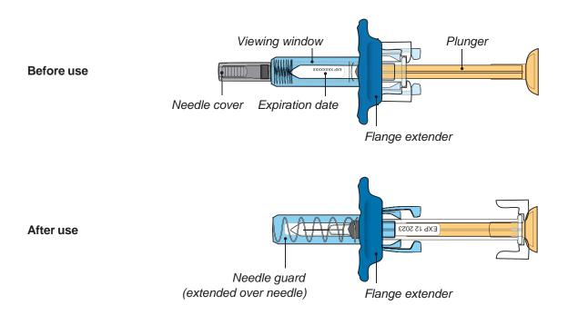
The prefilled syringe has a **flange extender** that makes it easier to hold and inject, and a **needle guard** that automatically covers the needle after a complete injection.
